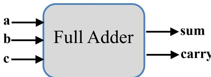
$$\begin{aligned} \text{sum}(a, b, c) &= a'b'c + a'bc' + ab'c' + abc \\ &= a \oplus b \oplus c \end{aligned}$$
